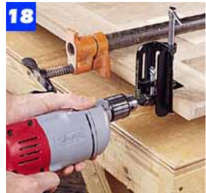
Clamp the breadboard end to the tabletop and use a doweling jig to bore through the strip into the end of the top.
