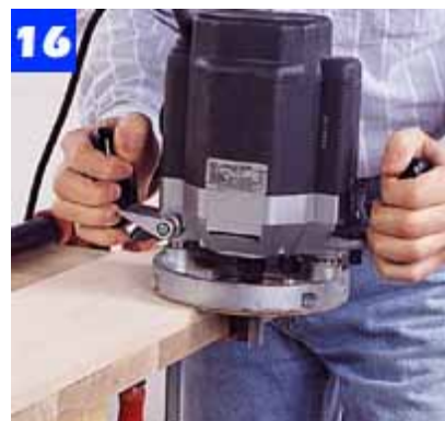
To trim the ends of the tabletop, use a template routing bit that follows a straightedge clamped to the workpiece.
