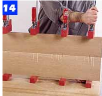
Begin assembly of the top by joining only two boards. After the glue cures, add one board at a time to reach full width.
